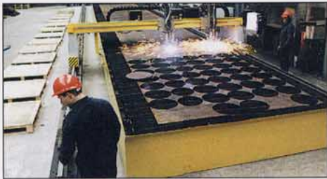
Profiling Machine, at Brown McFarlanes Warehouse
